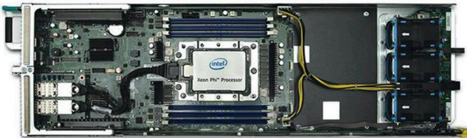
The 72-core, Knights Landing, Xeon Phi chip is available with built-in OmniPath fabric interfaces. The Groveport platform supports the Xeon Phi as a host processor.
